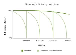
A standard solution using activated carbon treatment is both costly and ineffective compared to our Nodora CAT. The high performance of Nodora CAT is due to the the advanced active material used, the material mix and the overall design making use of all filter material equally. The experiments were conducted in Stockholm, with the collaboration of KTH Royal Institute of Technology. Real biogas conditions were tested with a  $H_2S$  concentration of 1000 ppm.
